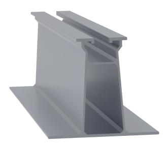
Height: 65mm Length: 300mm | Customised as per Crest Distance Raw Material Used: Aluminium 6063 T6 Certifications: TUV Certified for Tensile Strength and Chemical Composition.
