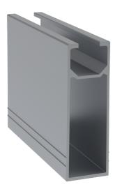
Height: 75mm Length: 100mm | 150mm | Customisable Raw Material Used: Aluminium 6063 T6 Certifications: TUV Certified for Tensile Strength and Chemical Composition.
