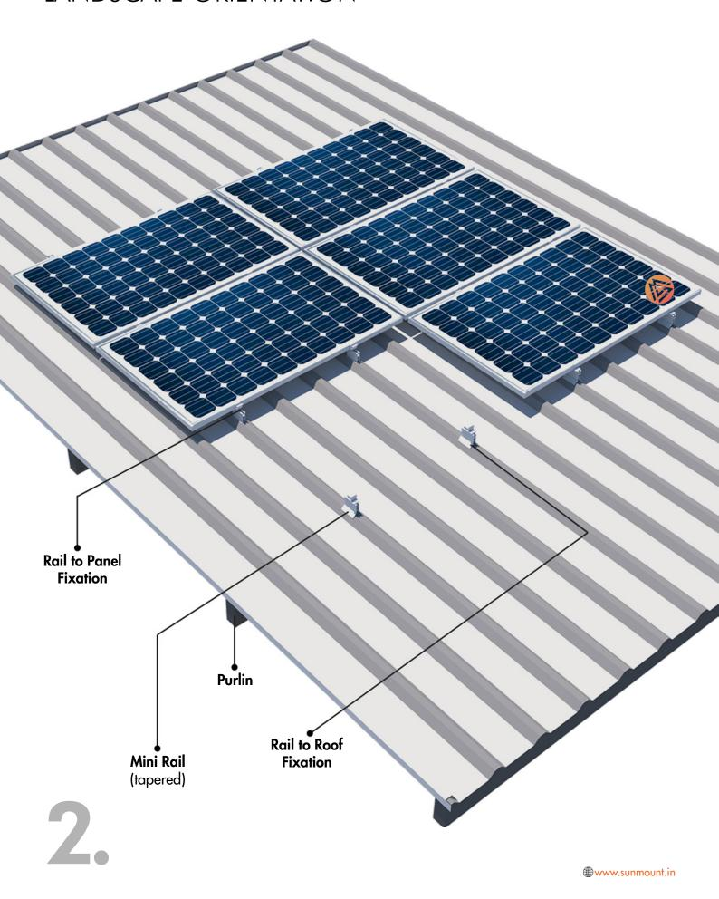
Mini Rail System is a lightweight and most optimum system for mounting solar PV panels on trapezoidal metal roof.
