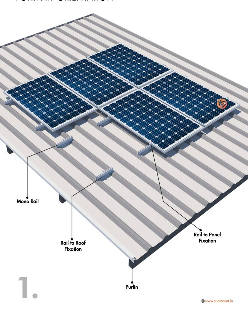
Mono Rail System is a lightweight and most optimum system for mounting solar PV panels on trapezoidal metal roof.
